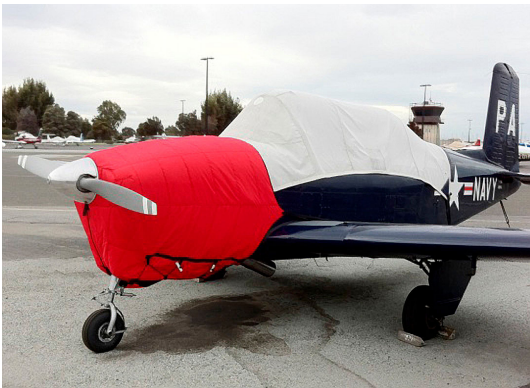
T-34A Insulated Engine Cover
