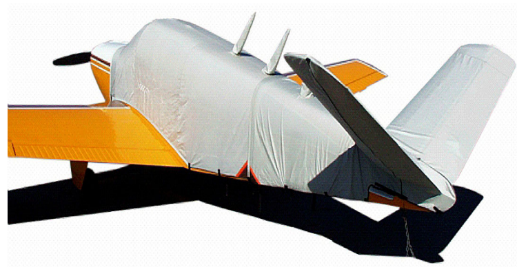
Extended Canopy Cover & Empennage Cover
