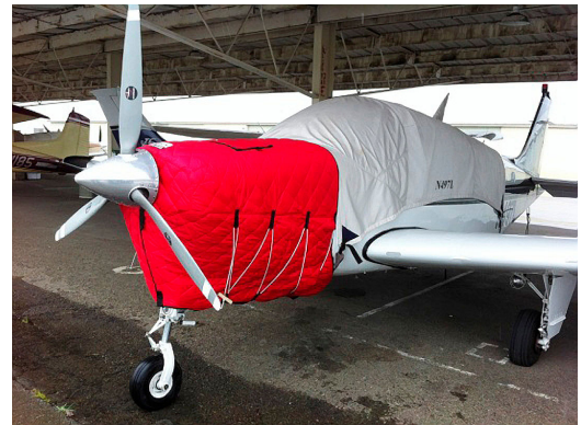
Beech Bonanza Insulated Engine Cover, fully enclosed
