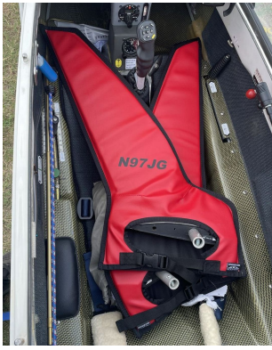
Schempp-Hirth Ventus-2B winglet/wingtip pads
