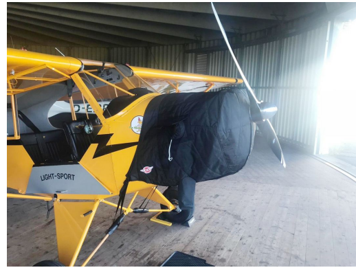
Legend Cub AL3 Insulated Engine Cover with special preheater access vent and attachment detail and fully enclosed under cowling.
