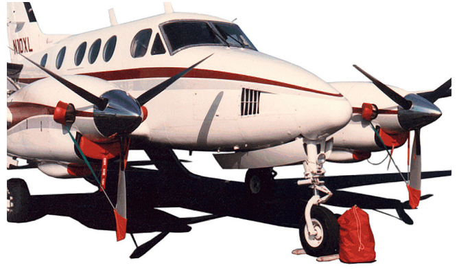
Pitot, Exhaust Covers, Engine Plugs & Prop Ties
