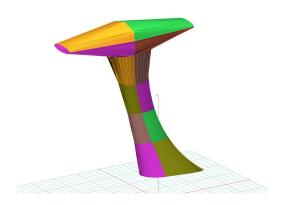
Autogyro Calidus Rotor Mast Cover, 3D model
