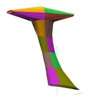
Autogyro Calidus Rotor Mast Cover, 3D model
