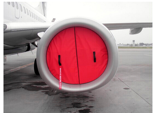
Boeing 737 Engine Intake Plug, Folding Type
