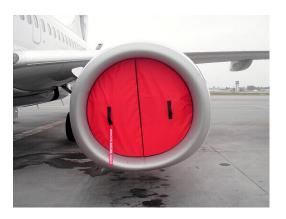
Boeing 737 Engine Intake Plug, Folding Type
