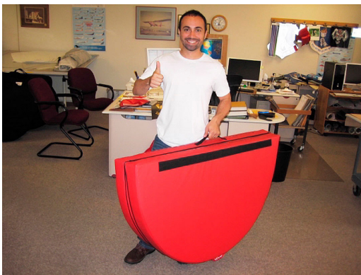
Boeing 737 FOD protection Intake Plug, folding type
