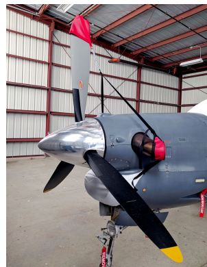
Embraer EMB 312 Tucano Prop Tie Down/Exhaust Covers
