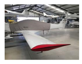
Dynaero MCR.4 Pickup Canopy Cover, Wingtip Pads
