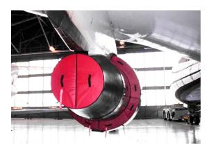
Exhaust Plugs Ship Set, incl. Fan Thrust Reverser and Exhaust Exhaust Plugs Ship Set, incl. Fan Thrust Reverser and Exhaust Plugs P/N: B767-200 Plugs P/N: B767-200
