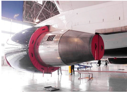
Exhaust Plugs Ship Set, incl. Fan Thrust Reverser and Exhaust Plugs P/N: B767-200 DC-10 Bypass Vent, Exhaust Plug set
