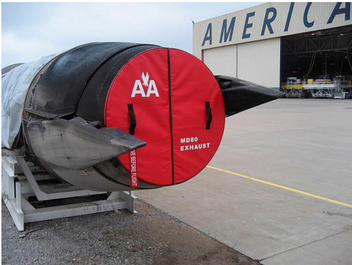
MD80 JT8D Exhaust Plug, Folding Type
