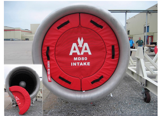
PW JT8D Off-Link Protective Long-term Storage "Rain Cap" Engine Cover MD-80 JT8D Intake Plug, mesh center & folding type
