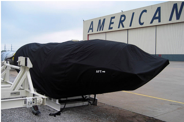
PW JT8D Off-Link Protective Long-term Storage "Rain Cap" Engine Cover MD-80 JT8D Intake Plug, mesh center & folding type
