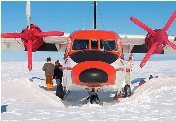
Casa 212 Insulated Engine & Propellor/Spinner Covers
