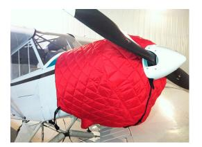
Piper Super Cub Insulated Engine Cover
