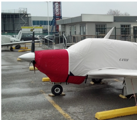
Mooney 201 Insulated Engine Cover, fully enclosed
