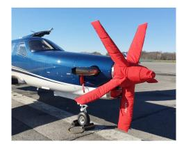
Socata TBM Insulated 5-Blade Prop/Spinner Cover
