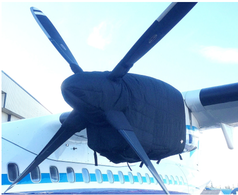
ATR-72-202 Insulated Engine & Prop Hub Covers
