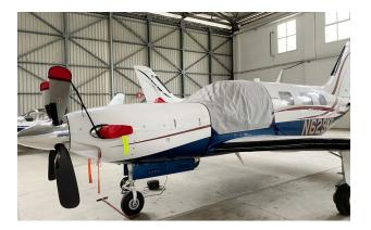
Piper PA-46-500TP Engine Cowling Top Plug
