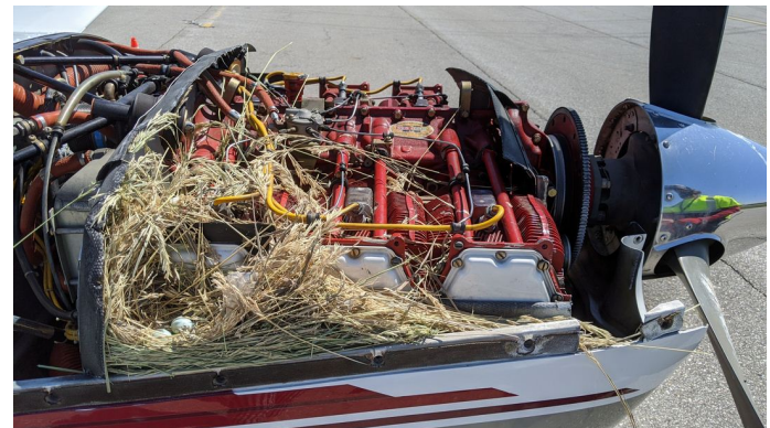
Piper PA-12 Wrap-Around Canopy Cover, Engine Plugs ENGINE PLUGS PREVENT BIRD NEST FOD. Piper Saratoga Engine Cowling Bird's Nest
