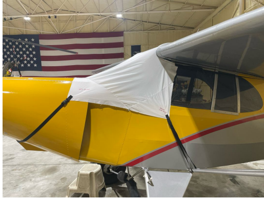
Piper J5A Windshield/Skylight Cover, test fit
