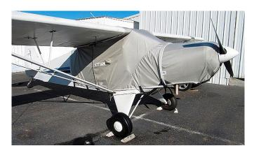
Piper Super Cub Insulated Engine Cover
