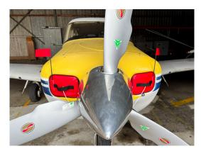
Piper PA-24-260 C Engine Inlet Plugs (set of 2)
