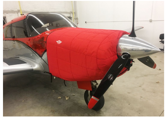
Piper Comanche Insulated Engine Cover, snap-on type
