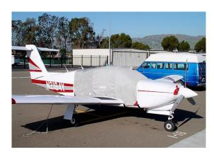
Piper PA-28 Turbo Arrow Extended Canopy Cover & Engine Inlet Plugs
