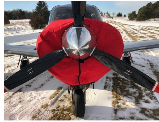
Piper Comanche PA-24 Insulated Engine Cover, snap-on type.
