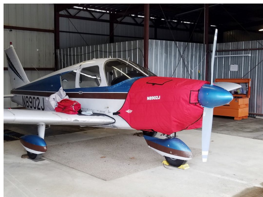
Piper PA-28 Insulated Engine Cover Piper PA-28-180 Insulated Engine Cover with Oil Filler Preheater Access and Inlet Preheater Access Ports Flaps
