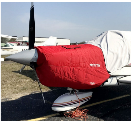
Piper PA-28 Insulated Engine Cover Piper PA-28-180 Insulated Engine Cover with Oil Filler Preheater Access and Inlet Preheater Access Ports Flaps
