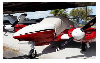
Piper Twin Comanche Canopy Cover, Wing & Engine Covers with Tip Tanks
