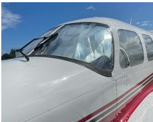
Piper PA-31 Models Cockpit HeatShields
