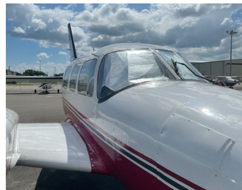
Piper PA-31 Models Cockpit HeatShields
