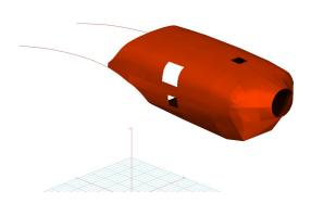
Piper Navajo Insulated Engine Cover, 3D model
