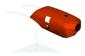
Piper Navajo Insulated Engine Cover, 3D model
