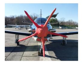
Socata TBM Insulated 5-Blade Prop/Spinner Cover
