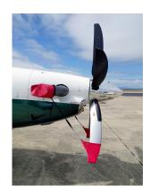
Pilatus PC-12 Prop Tie-Down/Exhaust Cover Set, 5 Blade
