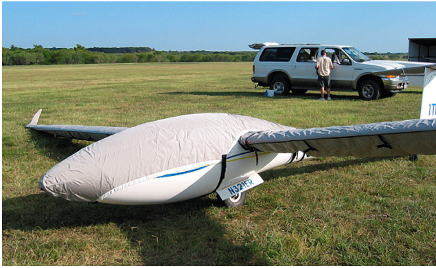
Canopy/Nose Cover, Wings and Horizontal Stab Covers
