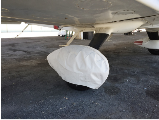
Grumman AA5 Main Wheelpant Cover, test fit
