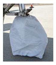
CJ1 Nose Gear Tire Cover, test fit
