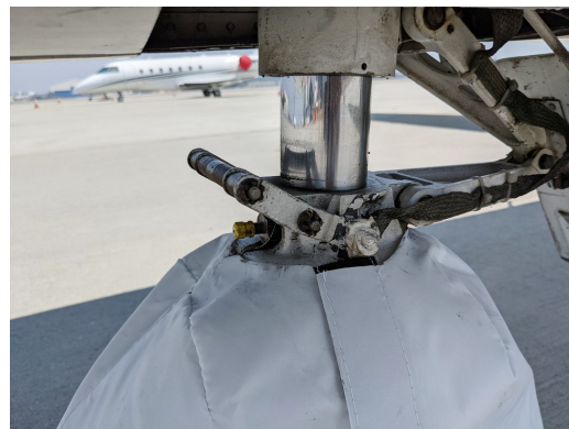
CJ1 Nose Gear Tire Cover, test fit
