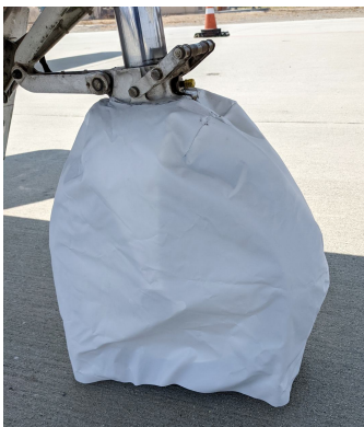
CJ1 Nose Gear Tire Cover, test fit
