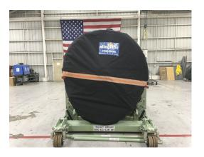
CFM56-5B Off Link Cover, fully enclosed
