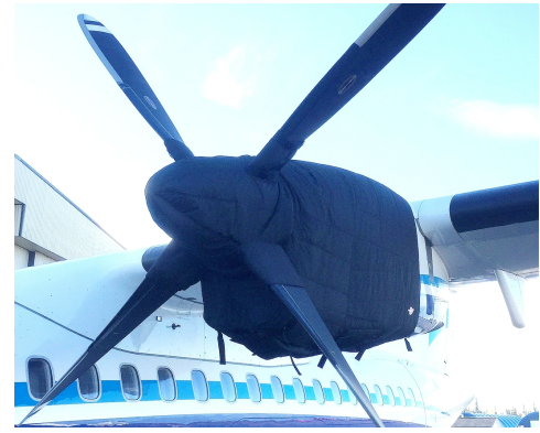
ATR-72-202 Insulated Engine & Prop Hub Covers
