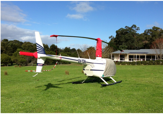
Robinson R-44 Bubble, Rotor Hub, Tail Rotor Covers, & Blade Tie-Downs
