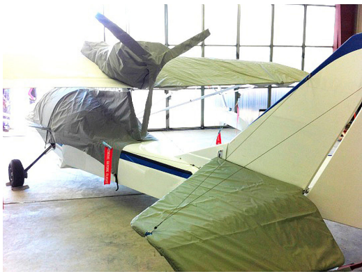
SeaRey Canopy, Engine, Wing & Horizontal Stab. (test fit covers)
