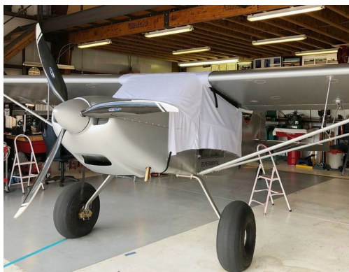
Rans S-20 Canopy Cover, test fit cover
