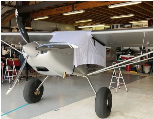
Rans S-20 Canopy Cover, test fit cover
