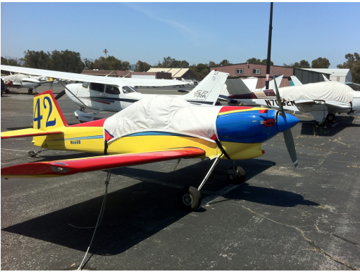
Vans's RV-3 Canopy Cover, Engine Plugs ENGINE PLUGS PREVENT BIRD NEST FOD. Piper Saratoga Engine Cowling Bird's Nest
