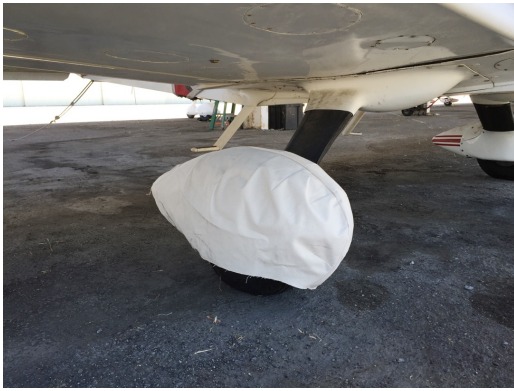
Grumman AA5 Main Wheelpant Cover, test fit
