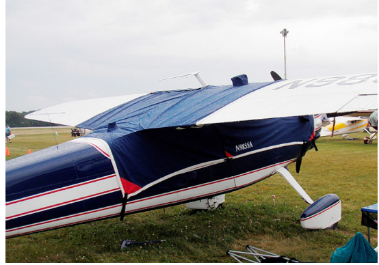
Cessna 195 Canopy Cover, extended forward and over gas caps Cessna 195 Canopy Cover, extended forward and over gas caps
