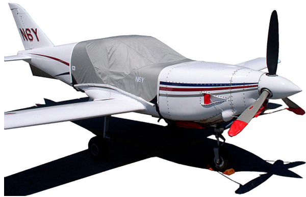
The Swearingen SX300 Canopy Cover, Engine Plugs & Prop Ties
