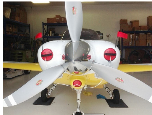
Swearingen SX300 Engine Inlet Plugs
