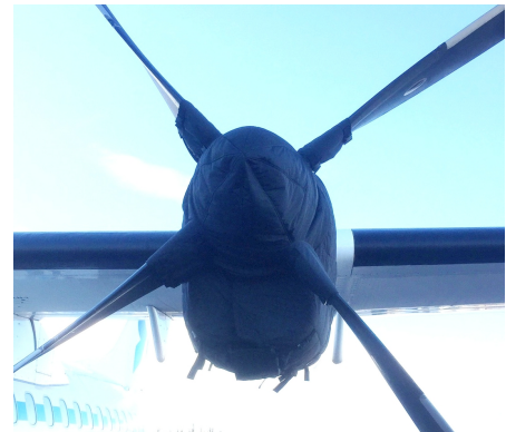
ATR-72-202 Insulated Engine & Prop Hub Covers
