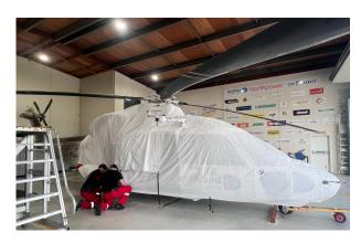
Sikorsky S76C Forward Canopy Cover, Engine Cover (test fit covers)
