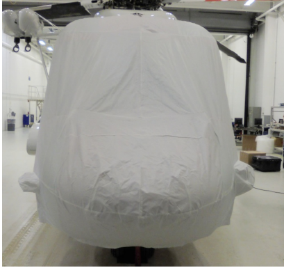
Sikorsky S-92 Windshield/Nose Cover, test fit cover
