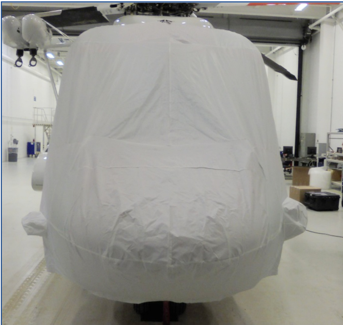
Sikorsky S-92 Windshield/Nose Cover, test fit cover
