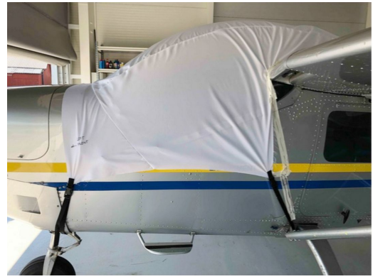
Saab Safari Canopy Cover, test fit cover
