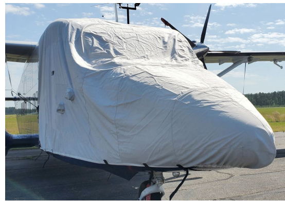
Short Skyvan Forward Fuselage/Nose Cover Short Brothers Sherpa, Skyvan, 330 & 360 (C-23) Forward Fuselage/Nose Cover
