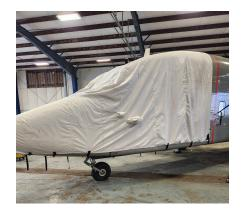
Short Brothers Sherpa, Skyvan, 330 & 360 (C-23) Forward Fuselage/Nose Cover Short Skyvan Forward Fuselage/Nose Cover
