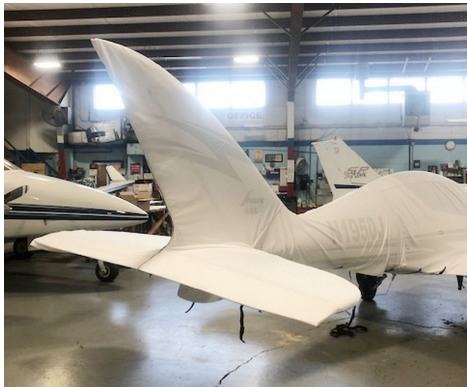
Shark 600 Complete Cover Set, test fit
