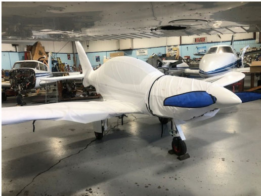
Shark 600 Complete Cover Set, test fit
