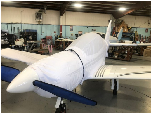
Shark 600 Complete Cover Set, test fit
