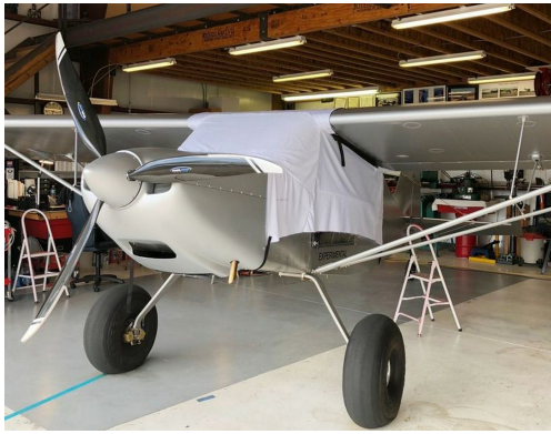
Rans S-20 Canopy Cover, test fit cover
