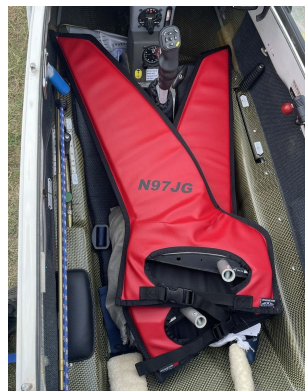
Schempp-Hirth Ventus-2B winglet/wingtip pads
