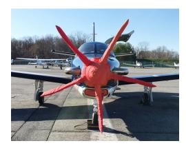
Socata TBM Insulated 5-Blade Prop/Spinner Cover
