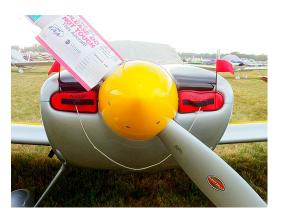
Vans's RV-7 Engine Engine Inlet Plugs
