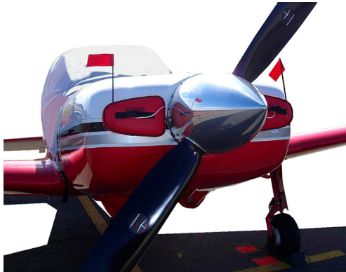
Micco SP20 Canopy Cover & Engine Inlet Plugs
