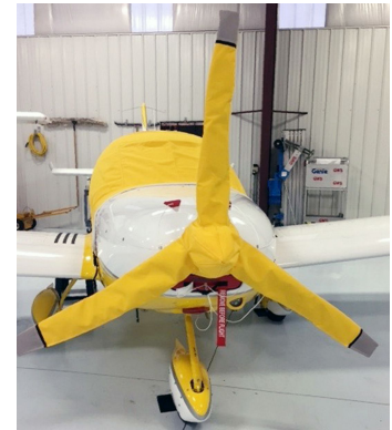
ENGINE PLUGS PREVENT BIRD NEST FOD. Piper Saratoga Engine Cowling Custom Yellow Canopy Cover, Prop/Spinner, and Inlet Plugs
