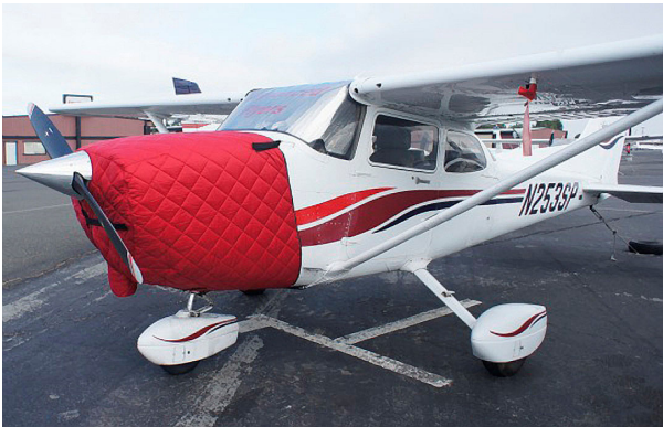
Cessna 172 Insulated Engine Cover, fully enclosed
