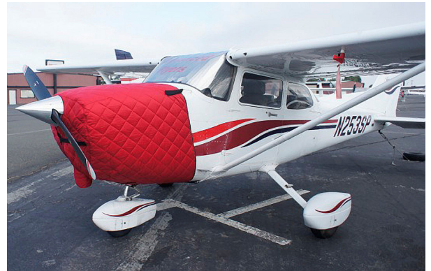
Cessna 172 Insulated Engine Cover, fully enclosed
