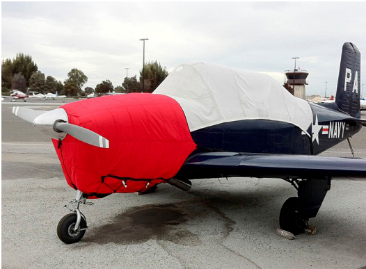
T-34A Insulated Engine Cover
